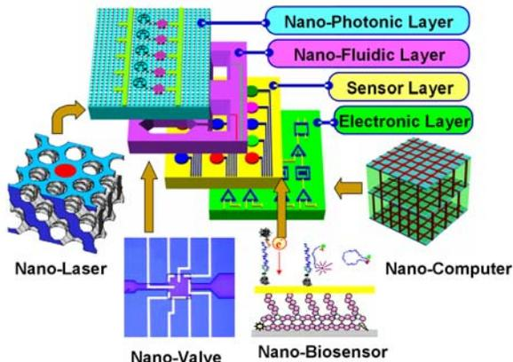
Conceptual schematic of a manufactured nanosystem
