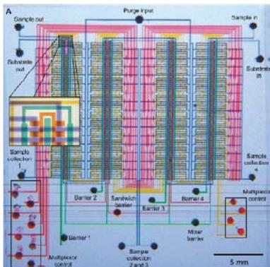
**Integrated circuits that are smaller and faster are possible with microfluidics systems built from or incorporating nanocomponents. At right is a microfluidic chip incorporating 2056 integrated valves in an area of one square inch (image courtesy of Thorsen et al.). NSF funding: Ferreira, 0328162, for the Center for Nano-Chemical-Electrical-Mechanical Manufacturing Systems.**
